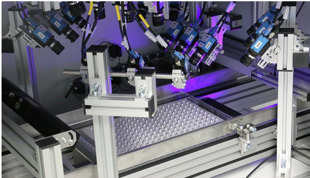
Fig. 01 Image data from IQZeProd's twenty TIS GigE industrial cameras as well as data from hyperspectral and non-optical sensors are fused using the Xeidana software framework to enable an inline QC system with zero errors. Image: Fraunhofer IWU ©
