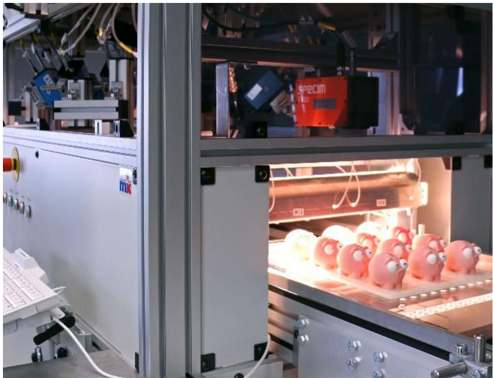
Fig. 03 Color testing of plastic toys with a hyperspectral line scan camera (type: Specim FX10). Image: Fraunhofer IWU ©
