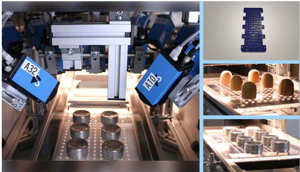
Fig. 05 Zoom cameras provide a rapidly adjustable field of view (FOV), allowing the demo system to scan components of diverse size and shape. Images: Fraunhofer IWU ©
