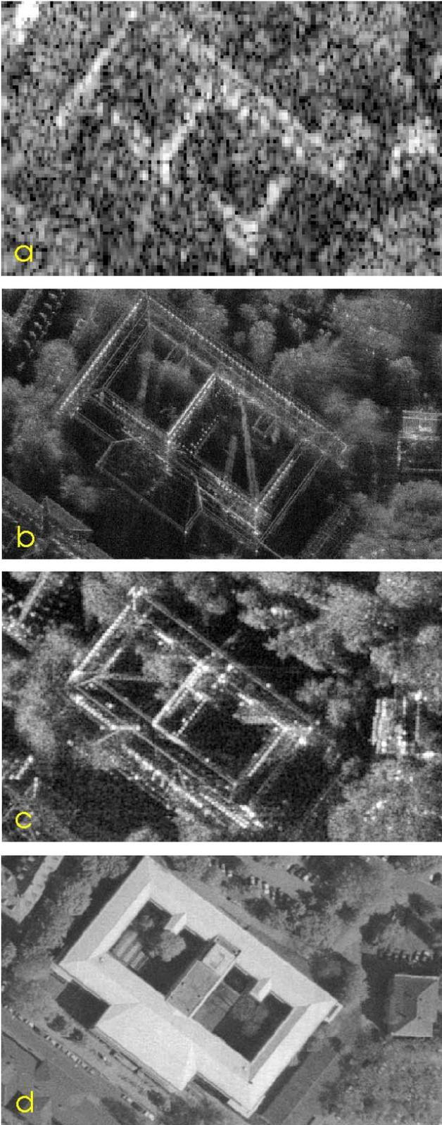
Figure 1. a) AER-II image with one meter resolution (range top-down), b) PAMIR image with resolution better than 20 cm (sliding spotlight mode, range top-down), c) PAMIR image with about 40 cm resolution (illumination from left), d) orthophoto (30cm)
