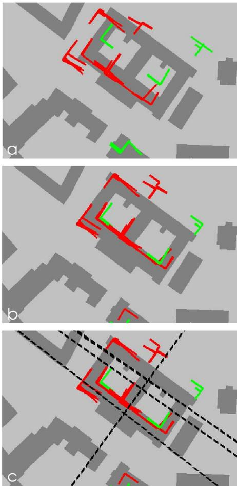
Figure 4. angle objects  $A_2$  used for assembly of symmetry objects  $S_y$ : a) before, b) after shift, c) like b) plus the detected symmetry axes (black).
