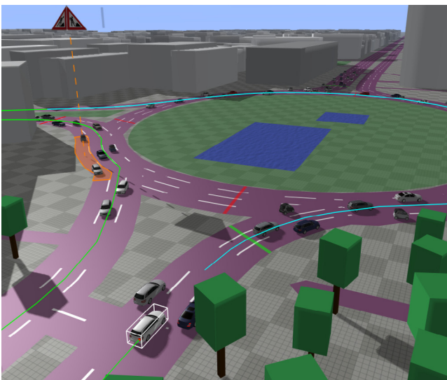
Figure 4: Simulator reference implementation – example scenario: Construction site at round about, Ernst-Reuter-Platz, Berlin, Germany
