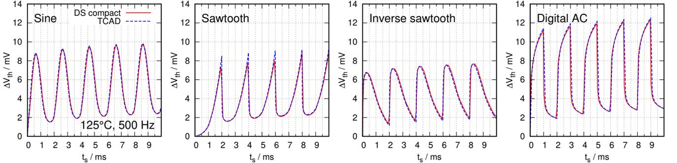
**Fig. 4:** Threshold voltage shift during analog stress. We compare the DS model results on  $\Delta V_{th}$  (solid line) to their TCAD reference (dashed line), for the first five periods of the stress phase. For all four stress patterns, both methods are in excellent agreement. The calculations use a stress frequency of 500Hz, a temperature of 125°C and voltage values  $V_l = 0.5$ V and  $V_h = 2.8$ V.
