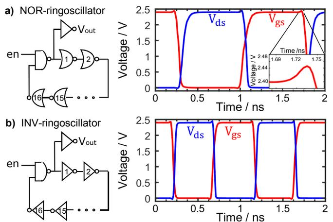
**Fig. 6:** Sketch of the schematic (left) and plot of the time-dependent pFET stress voltages  $V_{gs}$ ,  $V_{ds}$  (right) for the 17-stages **a)** inverter ring-oscillator and **b)** NOR ring-oscillator. The inset in the top-right plot shows the voltage overshoot in the oscillation pattern.
