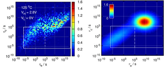
**Fig. 2:** Visualization of the CET maps in the NBTI defect sampling model (left) and the approach of fitting to a CET map ansatz function (right). The dimension of the z axis is mV. The white rectangles mark the windows of experimental characterization.
