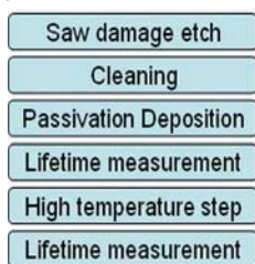
Figure 2. The lifetime samples were prepared following this depicted procedure.
