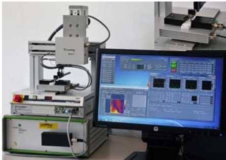
Fig. 1: Barkhausen Noise and Eddy current Microscope (BEMI II) and detail of BEMI probe (upper right)
