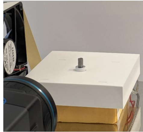
Figure 2: Propellant grain placed on the insulated fixture in front of the IR camera.
