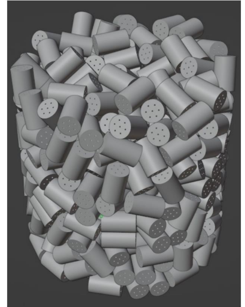
Simulated bed of JA2 propellant grains in a 700 cm 3 vessel with transparent walls [3].
