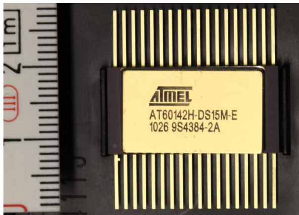
Fig. 9. Photo of the selected type of SRAM for the detection of solar particles.
