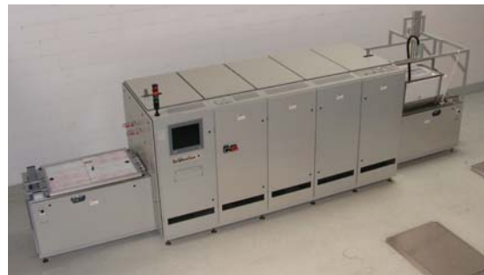
Figure 1: Inline annealing furnace located at Fraunhofer ISE. The system was built by centrotherm photovoltaics AG.
