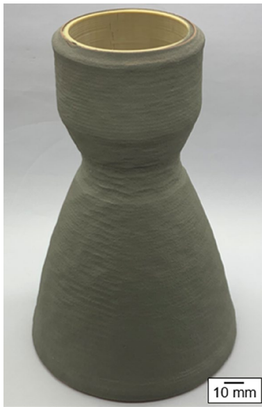
Fig. 11 Sprayed rocket liner on PEEK mold
