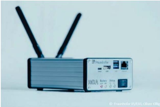
Figure 4. Prototype of the Wireless Network Monitoring node of Fraunhofer IIS/EAS as tool for permanent monitoring and diagnostic of industrial wireless networks
