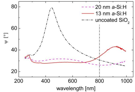
**Fig. 3:** Measured  $\psi$  values for an 13 and 20 nm thick *a*-Si:H layer deposited on a 105 nm thermally grown SiO<sub>2</sub> layer compared to the data measured on the uncoated SiO<sub>2</sub> layer.  $\psi$  data is shown for an angle of incidence of 70°.
