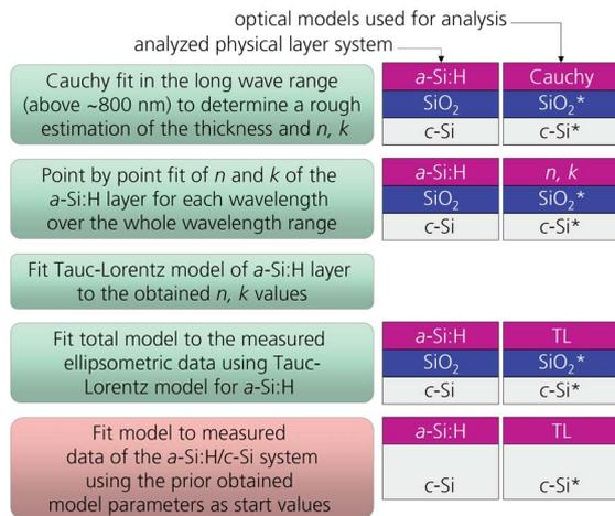
**Fig. 4:** Flow chart of the fitting procedure for ultrathin *a*-Si:H layers. The applied layer structure and the used optical model are shown on the right. Layers marked with a \* are model by tabulated data.
