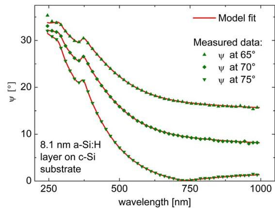
**Fig. 5:** Measured and modeled ellipsometric data of a 8.1 nm thick *a*-Si:H layer on *c*-Si substrate. Data is shown for different angles of incidence. Modeling has been done corresponding to the presented modeling procedure. A very good agreement between measured and modeled data is obtained.
