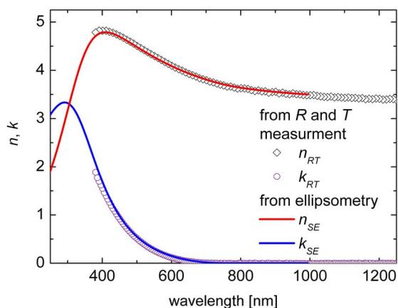
**Fig. 6:** Comparison of  $n$  and  $k$  for a 8.1 nm thick  $a$ -Si:H layer obtained from ellipsometry and RT analysis. The ellipsometry analysis was performed for an  $a$ -Si:H layer on  $c$ -Si substrate, the RT analysis for an  $a$ -Si:H layer on glass substrate. Both layers were deposited simultaneously.
