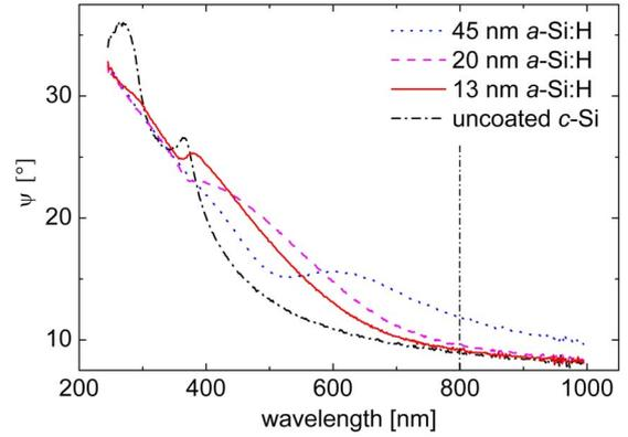
**Fig. 2:** Measured  $\psi$  values for an 13, 20 and 45 nm thick *a*-Si:H layer deposited on *c*-Si substrate compared to the data measured on uncoated *c*-Si. In this case  $\psi$  is measured at an angle of incidence of 70°.
