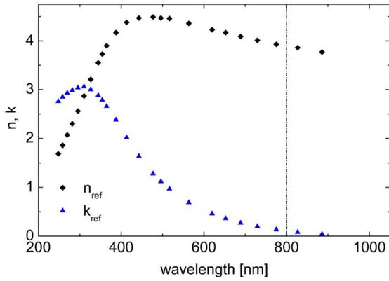
**Fig. 1:** Refractive index  $n_{ref}$  and extinction coefficient  $k_{ref}$  of amorphous silicon according to Ref. 10.
