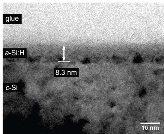
**Fig. 7:** TEM micrograph of the 8 nm thick  $a$ -Si:H layer deposited  $c$ -Si. Due to the TEM sample preparation there is glue on top of the  $a$ -Si:H layer. With the ellipsometric analysis a layer thickness of 8.1 nm was obtained.
