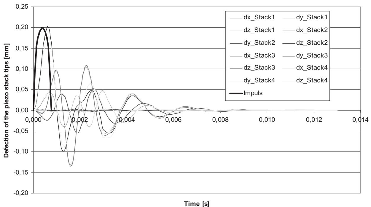
**Figure 8:** Transient dynamic behaviour of NGV test-bench clamping platform with piezo-stacks
