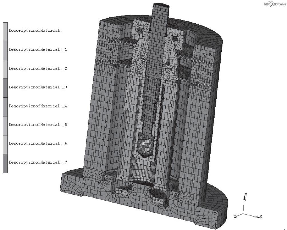
**Figure 4:** The FE model of the piezoelectric clamping module (cross section)
