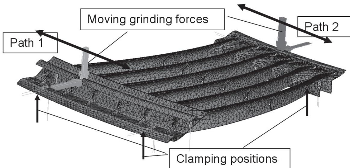
**Figure 6:** FE model with fixed clamping positions and moving grinding forces
