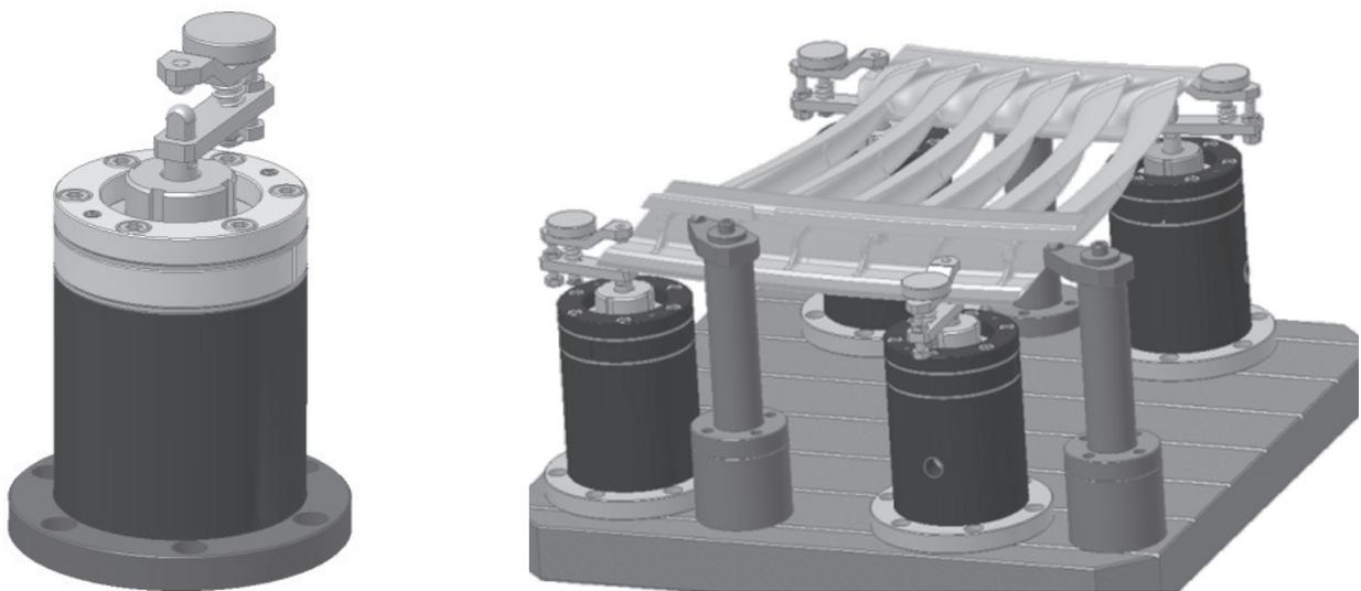
**Figure 2:** *The adaptive clamping module and the complete fixture platform with the clamping modules*
