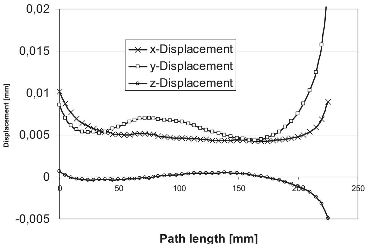
**Figure 7:** Displacement of the contact point between wheel and NGV when grinding the inner perpendicular surface along path 1
