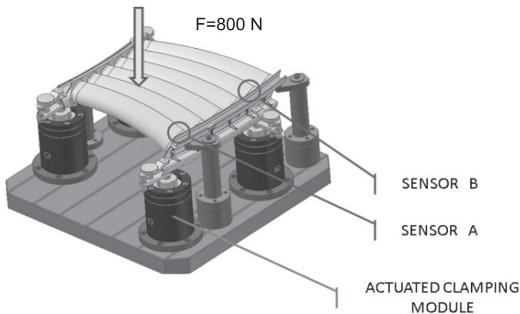
**Figure 9:** Layout of the open loop test with an applied force
