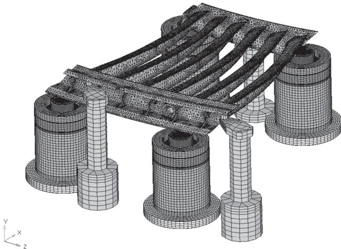
**Figure 5:** FE model of the test-bench fixture platform with the mounted NGV
