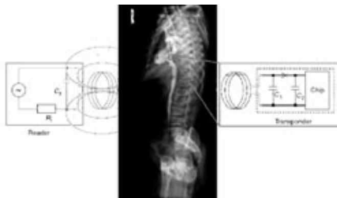
Figure 1: Model of an inductive sensor transponder system for medical applications (X-ray picture: Deutsches Röntgen-Museum)
