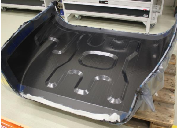
Figure 11. Generic shell wet panel on curing tool after transfer (left); cured generic shell part (right)
