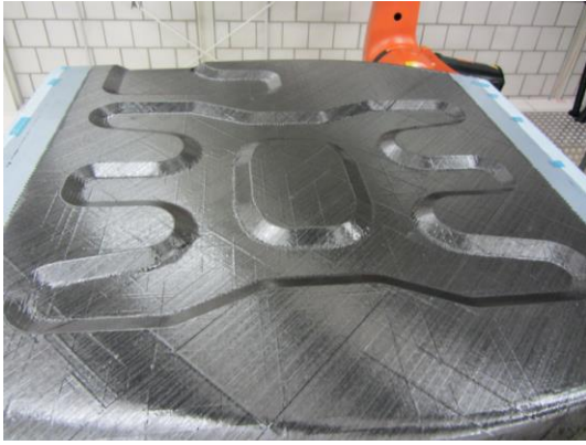
Figure 9. AFP layup of the generic shell part: inner skin (left), outer skin (right)
