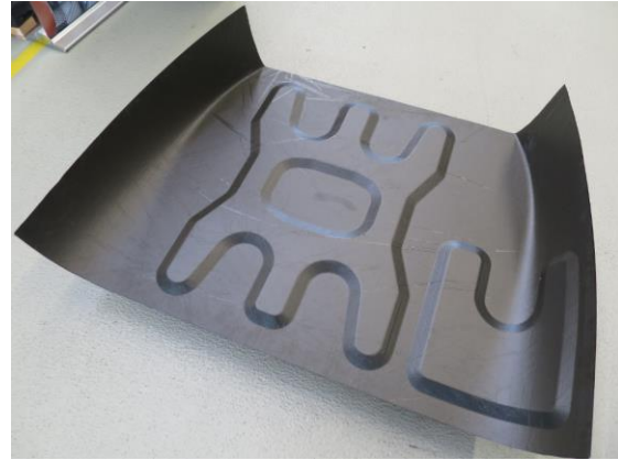
Figure 11. Generic shell wet panel on curing tool after transfer (left); cured generic shell part (right)
