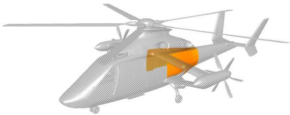
Figure 1. Digital mock-up of RACER IDP; focused sideshell parts are highlighted
