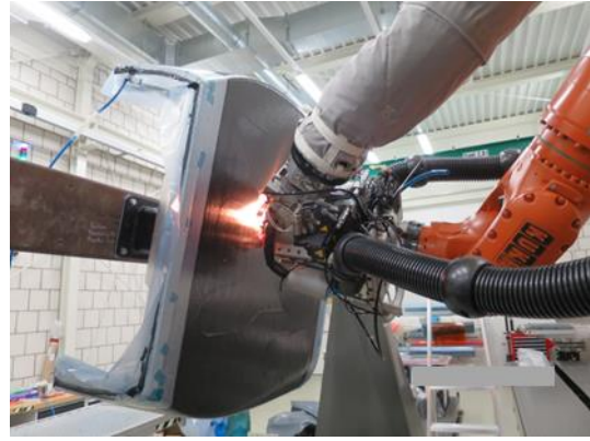
Figure 9. AFP layup of the generic shell part: inner skin (left), outer skin (right)
