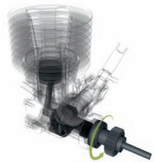
Moving two-stroke engine including views of the CT recording. Photo: Fraunhofer IIS
