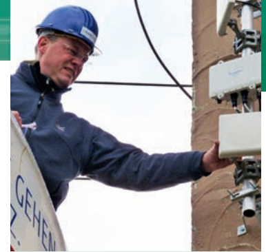
A researcher adjusts the antennas of the WiBACK system. Photo: Fraunhofer FOKUS
