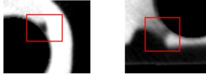
Figure 3. Part of a slice view extracted from a 3D-CT volume: on the left side a true defect (surface defect) appears as a darker area and on the right side a false alarm (reconstruction artefact) appears as a darker area as well.
