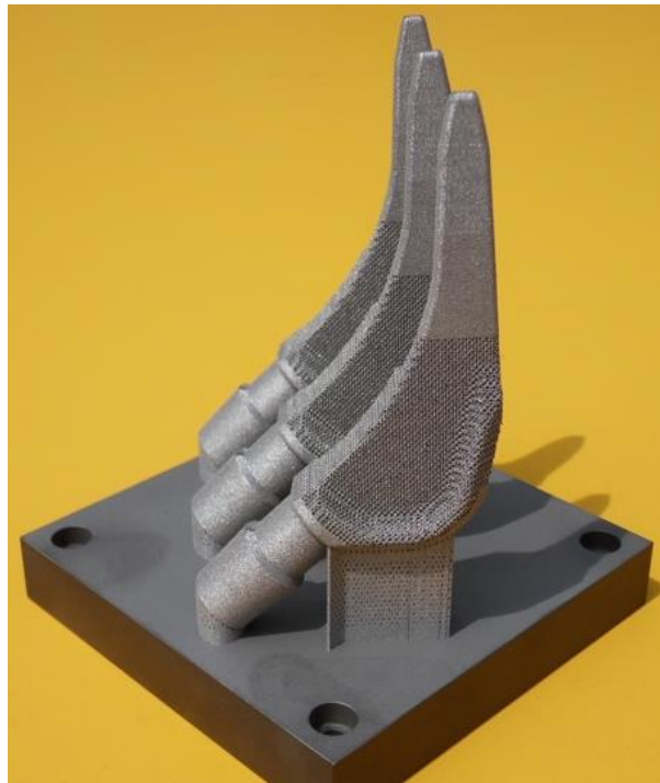
Laser beam melted implants on build platform
