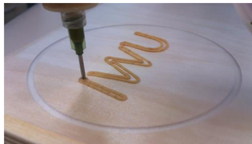
successful printing test, considering the visco-elastic behavior of paste
