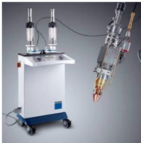
Laser deposition welding DepositionLine + TruDisk 6002 (Trumpf), IWU Chemnitz
