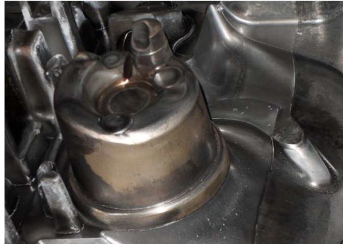
tooling insert with conformal cooling
