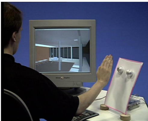
Fig.5. Setup of the system of EFSs for navigation in virtual environments.
