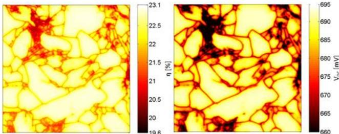
Fig. 3: Predicted local efficiency  $\eta$  and  $V_{OC}$  for a lifetime sample with designated cell design.
