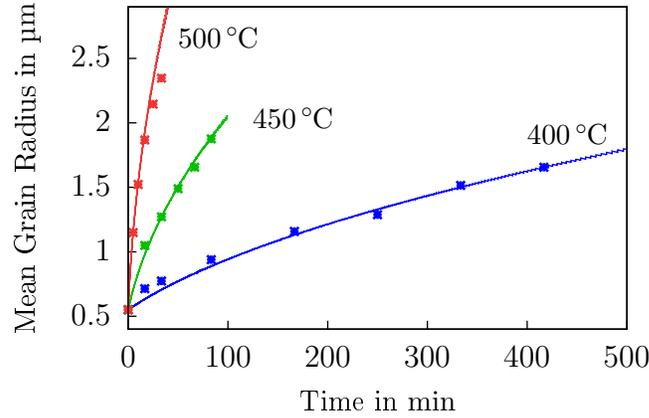
**Figure 3.** Mean radius evolution for 1000 two-dimensional grains with Hillert's distribution for two dimensions with  $\sigma = 0.625 \text{ J/m}^2$ ,  $Q = 154 \text{ kJ/mol}$ ,  $M_0 = 5.6 \cdot 10^{-4} \text{ m}^4/(\text{Js})$ . Experimental data from [38].
