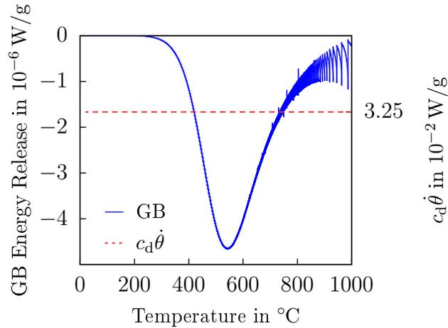
**Figure 5.** Comparison of the two contributions to the heat supply in the virtual calorimetry experiment. Note the opposed signs and different orders of magnitude.
