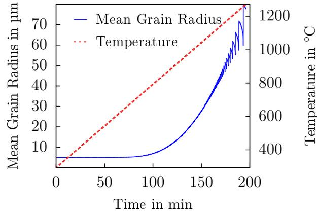
**Figure 4.** Temperature ramp applied in the virtual calorimetry experiment and resulting evolution of the mean grain size.
