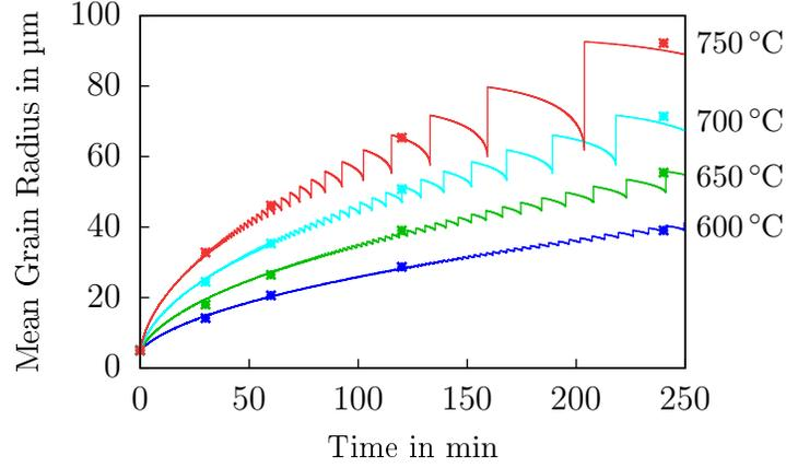
**Figure 2.** Mean radius evolution for 10 000 grains with Hillert's distribution,  $\sigma = 0.625 \text{ J/m}^2$ ,  $Q = 82 \text{ kJ/mol}$ ,  $M_0 = 3.5 \cdot 10^{-8} \text{ m}^4/(\text{Js})$ . Experimental data from [37].
