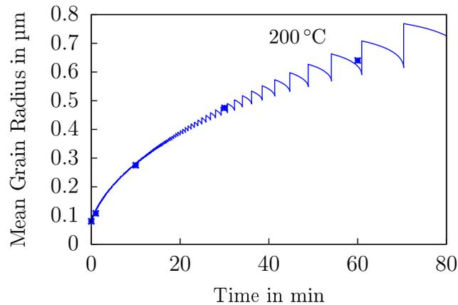
**Figure 1.** Mean radius evolution for 3000 grains with Hillert's distribution,  $\sigma = 0.625 \text{ J/m}^2$ ,  $Q = 102 \text{ kJ/mol}$ ,  $M_0 = 9.0 \cdot 10^{-5} \text{ m}^4/(\text{J s})$ . Experimental data from [36].
