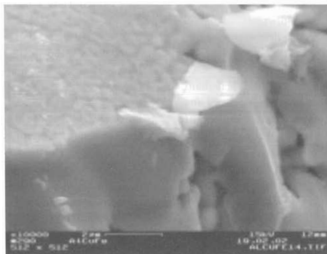
Figure 13. SEM exposure of a fiber break edge of an AlCuFe fiber before the ODH of propane.
