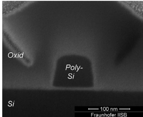
Fig. 6. SEM cross section image of a poly-Si gate, patterned by UV NIL and RIE. The channel length is around 90 nm.
