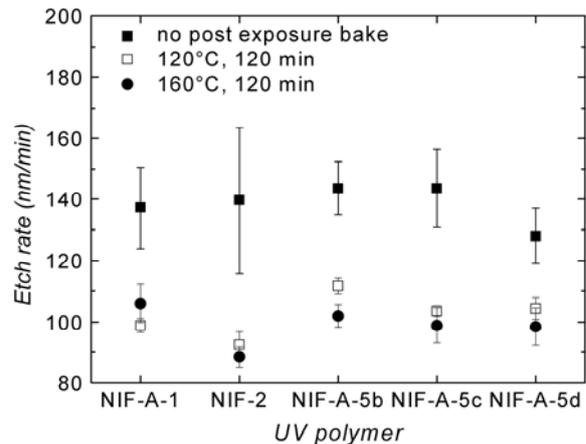
Fig. 3. UV polymer etch rates for different post exposure bake conditions against the RLT etching process.
