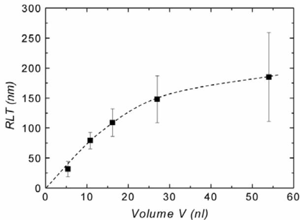
Fig. 1. Residual layer thickness for different amounts of dispensed UV polymer NIF-A-5b.
