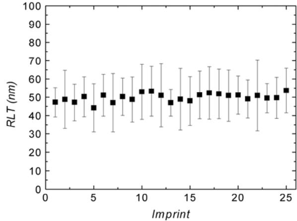
Fig. 2. Residual layer thickness for 25 imprints on a Si substrate. The resist used was NIF-A-5b.
