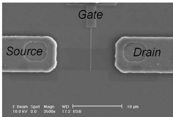
Fig. 5. SEM top view image of the fabricated short channel n-MOSFET.
