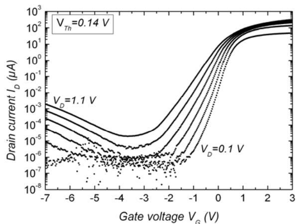
Fig. 7. Transfer characteristic of the short channel n-MOSFET shown in Fig. 6 with a channel length of about 90 nm.
