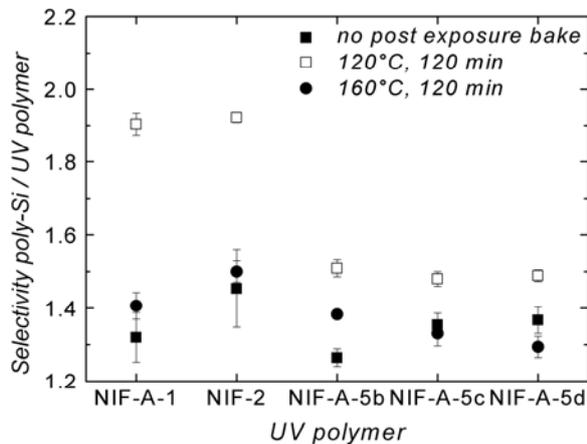
Fig. 4. UV polymer etch resistance for different post exposure bake conditions against the poly-Si etch process.
