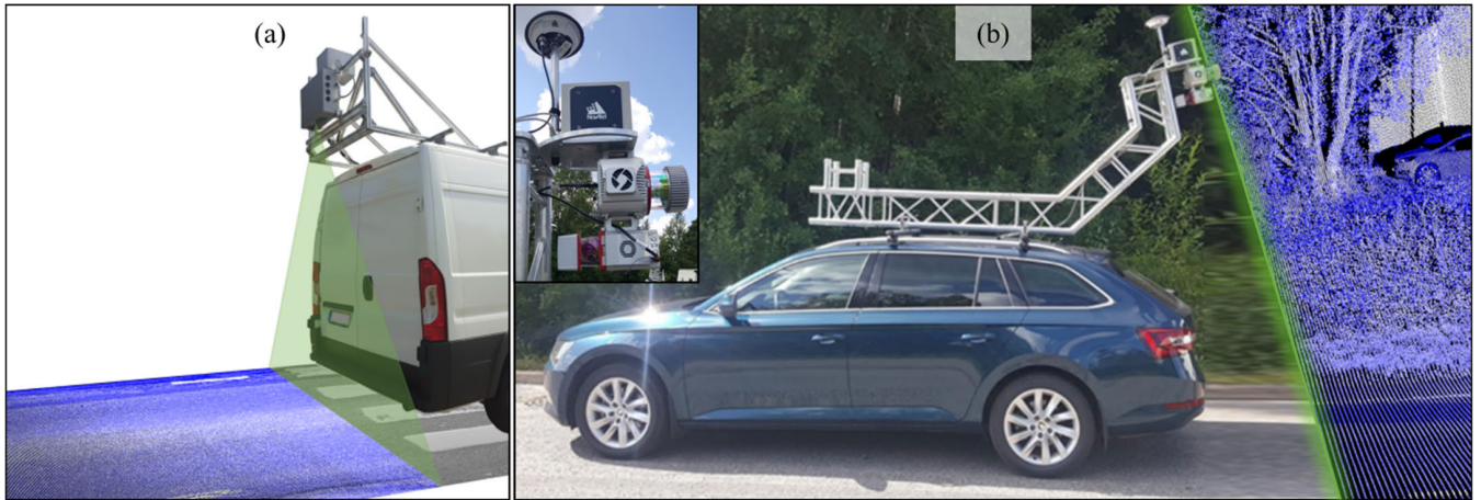
FIGURE 2. Fraunhofer PPS-plus reference system, illustrating its scan angle (green) and the resulting dense pavement point cloud (blue) on the road surface. (b) The Roamer-R4DW conventional MLS system, which captures the entire road environment with a 360-degree scanner (green line and blue point cloud), resulting in a comparatively sparser point cloud on the road surface; the inset provides a close-up of the sensor setup. (Fig. 2. (b) modified from [21], ©2021 by the authors. Licensed under CC BY 4.0).
