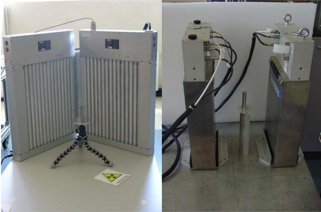
**Figure 2:** Measurement set-up of the Fission Meter (left) and of the Slab Counters (right). The distance of the source on the tripod to the center of one of the Fission Meter panels was 24 cm. The distance between the front surfaces of the Slabs was 23 cm
