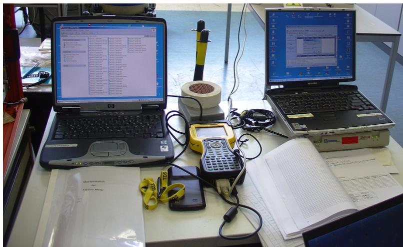
**Figure 3:** The Fission Meter data collection device (in the center of the picture), the Slab Counter high voltage supply and data collection unit (right, beneath the notebook) and notebooks.
