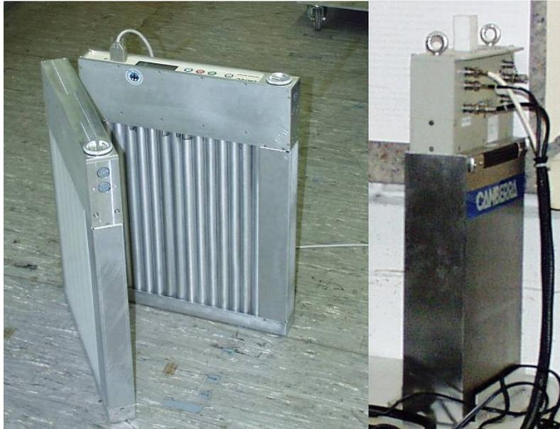
**Figure 1:** Detection panels of the Fission Meter (left) and the Slab Counter (right).
