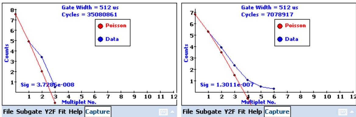
**Figure 3:** Multiplicity plots of the Fission Meter for a background measurement (left) and with the source Pu CBNM 61 (right).
