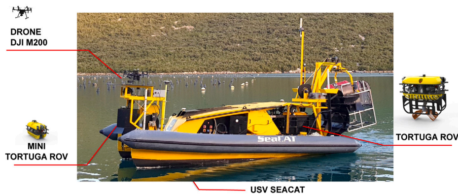
(b) Modules when loaded on the SeaCat USV.
