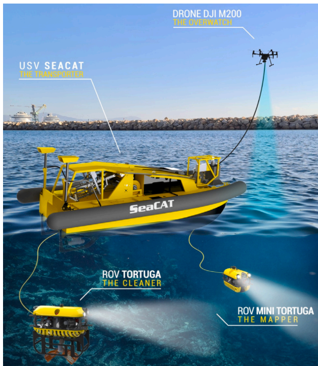
Fig. 1. Overview of the SeaClear robotic platform.
