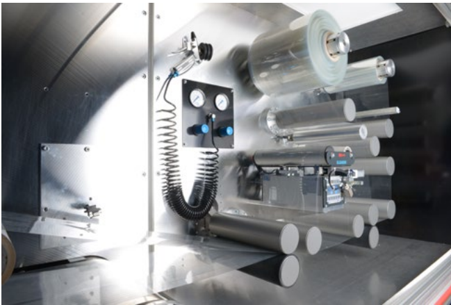
Figure 16: Production of microfluidic structured films using a roll-to-roll process.
