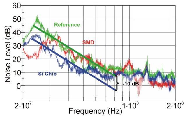
Fig. 9. Comparison of electromagnetic behavior of one phase of an module with silicon chip snubber to SMD snubber and without snubber
