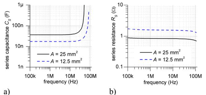
Fig. 6. a) Capacitance and b) resistance of diced RC-snubbers with a device area of 12.5 mm<sup>2</sup> and 25 mm<sup>2</sup> over a frequency range of 100 kHz to 110 MHz
