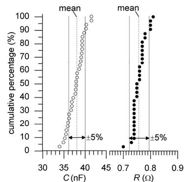
Fig. 3. Cumulative percentage of the capacitance and of the resistance for 33 RC-snubber with an area of 25 mm<sup>2</sup> over a 150 mm wafer
