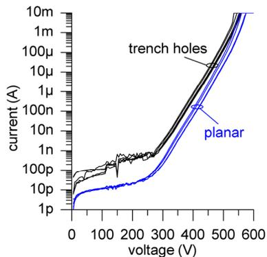
Fig. 5. I-V curves of planar and trench RC-snubbers with an device area of 1 mm<sup>2</sup>
