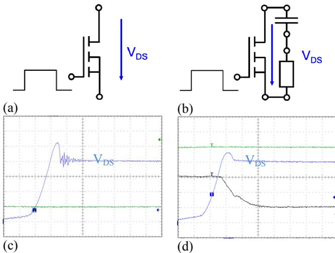
Fig. 8. MOS power switch a) without snubber, b) with RC snubber; simulated time dependent voltage during switching c) without snubber, d) with silicon chip snubber
