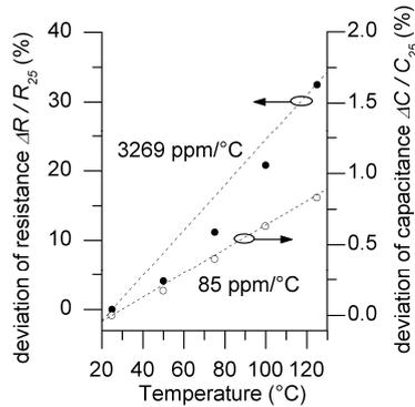
Fig. 4. Temperature dependent deviation of the capacitance ( $\Delta C$ ) and the resistance ( $\Delta R$ ) normalized to the values at 25°C ( $C_{25}$ ,  $R_{25}$ ), for temperatures between 25°C and 125°C
