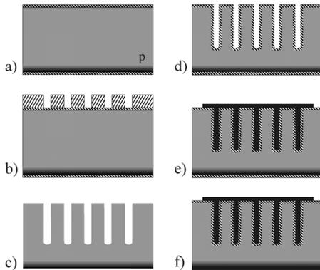
Fig. 2. Simplified process flow for a monolithic RC-snubber. a) thermal oxidation, back side doping and annealing, b) first lithography of the trenches, c) dry etching and removal of the photo resist and SiO<sub>2</sub>, d) processing of the dielectric stack, e) processing and patterning the top electrode, f) cleaning of back side and processing the bottom electrode
