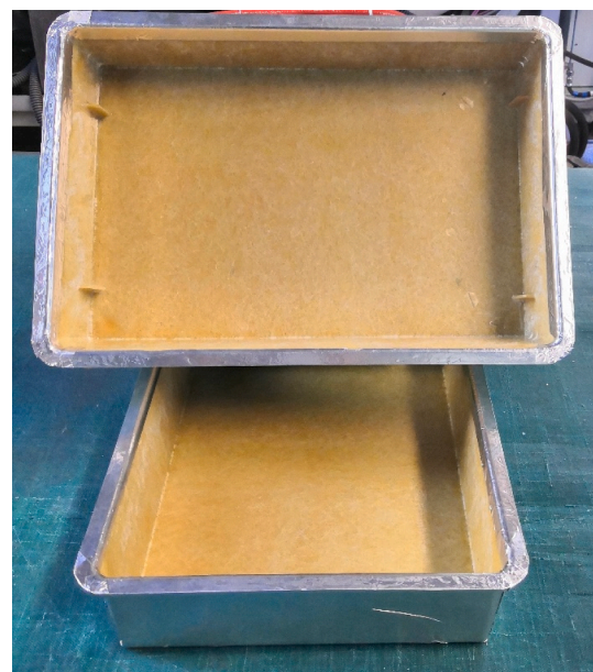
Fig. 1. Two halves of the composite test housing made of UPPH-GF40 covered with aluminium foil.
