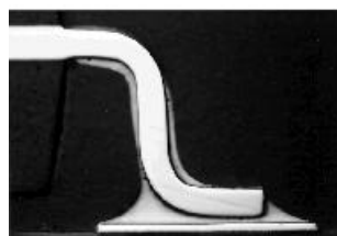
Fig. 3.4: Soldering of SMD chips with diode lasers
