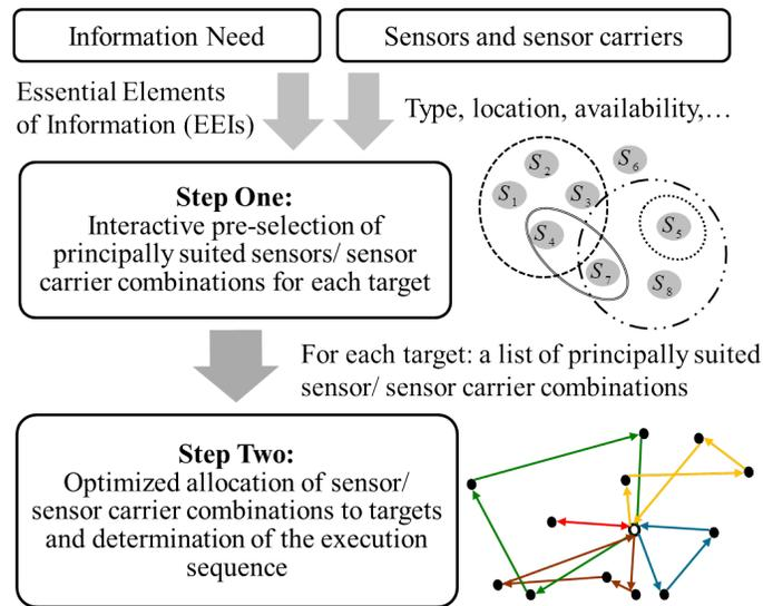
Fig. 2. Schematic illustration of the two-step approach for resource-optimal sensor scheduling. At Step One, for each target, the set of available assets ( $S$ ) being principally suited according to certain selection criteria is determined sequentially. Step Two aims to derive concrete proposals which assets have to be finally assigned to which targets and the dedicated routes individual assets have to follow in order to serve these targets.
