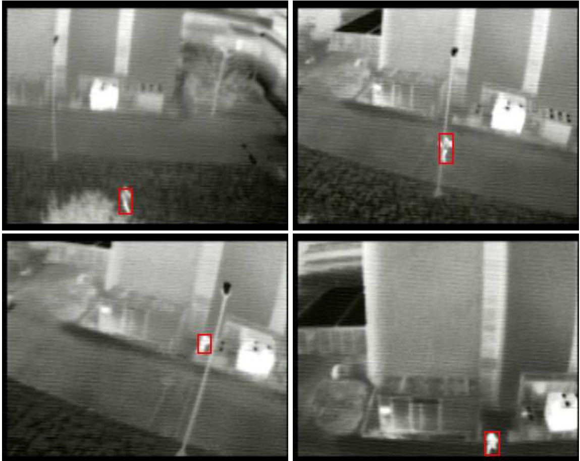
Figure 4. Tracking a suspicious running person with a thermal infrared camera mounted on a security quadcopter.
