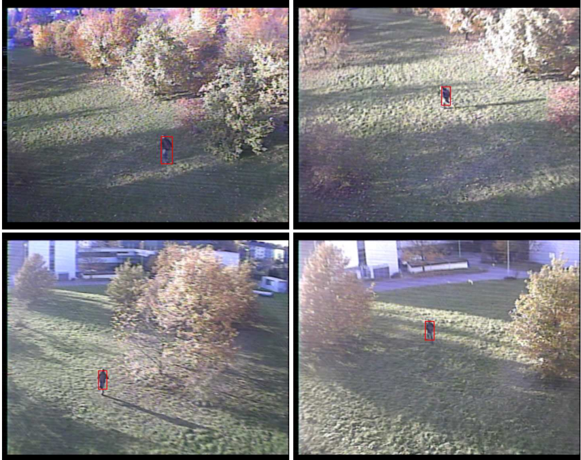
Figure 3. Tracking a suspicious running person with a visual-optical camera mounted on a security quadcopter. Four single images are picked out of the sequence and depicted here to represent the tracking results for the sequence.
