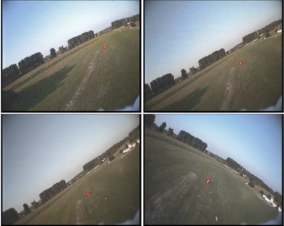
Figure 6. Tracking a target on a grassland with a UAV using an analog on board camera using PAL resolution (in the control loop PAL/4 is used, see text).
