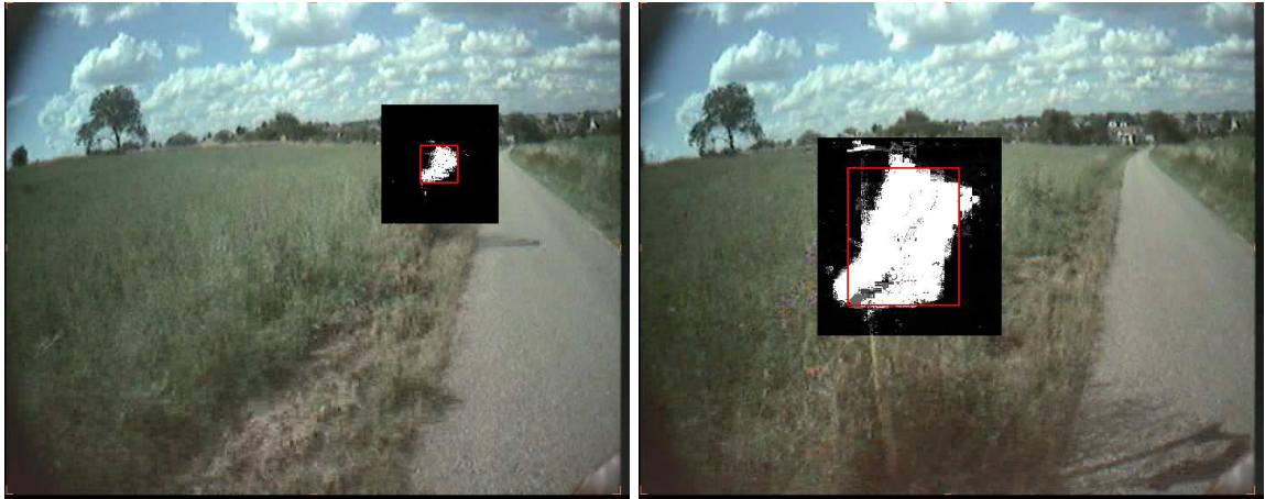
Figure 2. Visualisation of the weighting function w^{(n)} for the two lower tracking results in Figure 1. w^{(n)} was applied on the colors of image i^{(n+1)} and displayed via overlaid grayvalues. The darker the pixels in the tracking region, the smaller is the color weight w^{(n)} . And the brighter they are, the more characteristic could the respective image colors be categorized.
