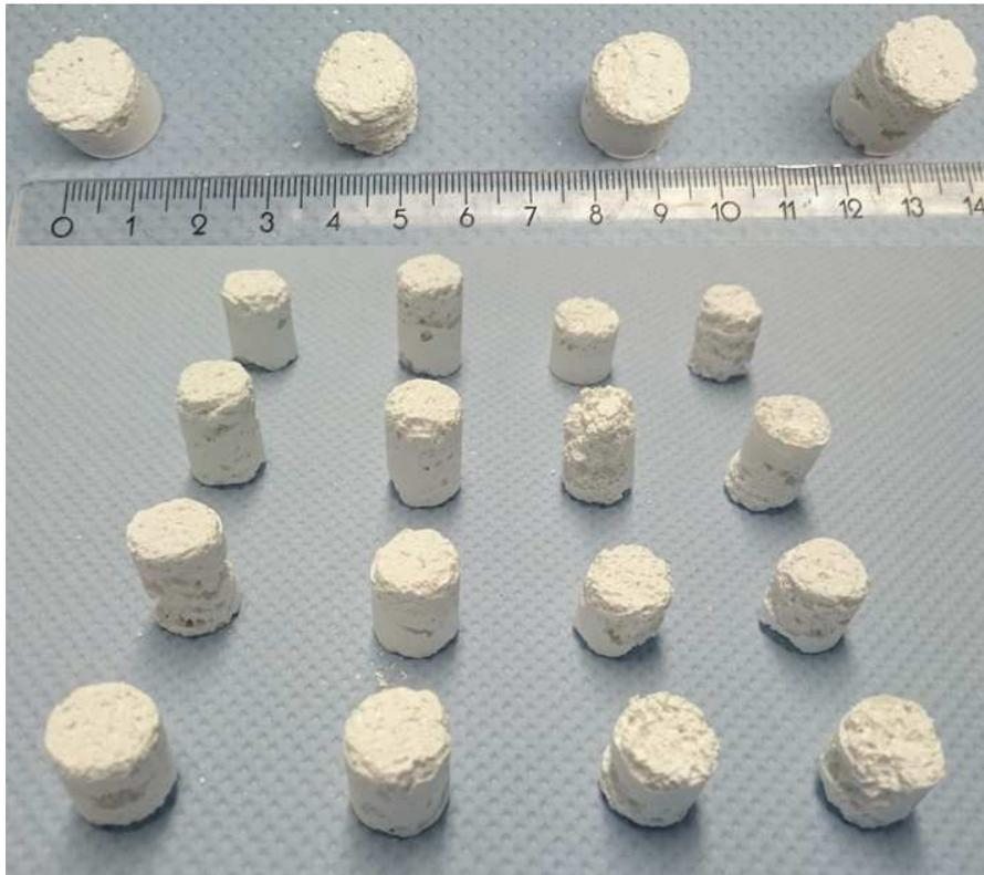
Figure 7. Manufactured model Freeze Foams (green state).
