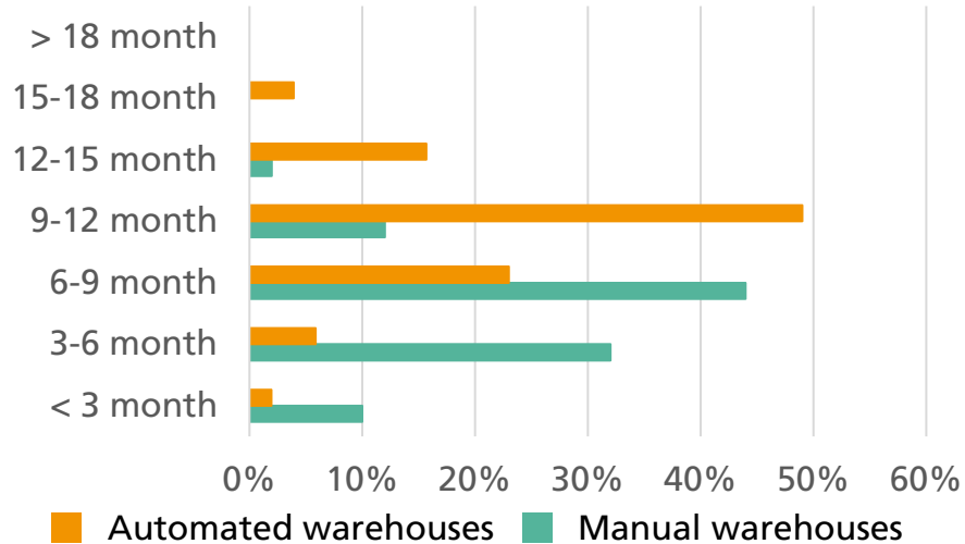
Ø Duration of a WMS Implementation for Manual and Automated Warehouses for New Customers
