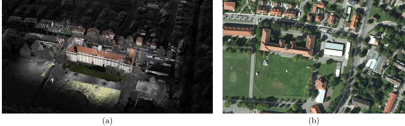
Figure 1. Background models for image based geo-referentiation - (a) Multiple jointly registered airborne and terrestrial LiDAR scans for low aspect UAV video streams. (b) Orthophoto mosaic representation for high altitude UAV video stream geo-referentiation.
