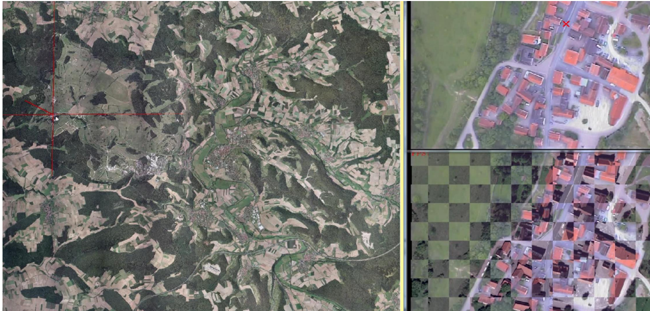
Figure 5. Visualization of the geo-referentiation system using high altitude UAV footage and Orthophotos as the underlying background model. The left image shows the orthophoto map with the geo-location of the marked pixel (red cross) in the video-stream (upper right image). The transfer is calculated by the registration of the model with the camera image (bottom-right).
