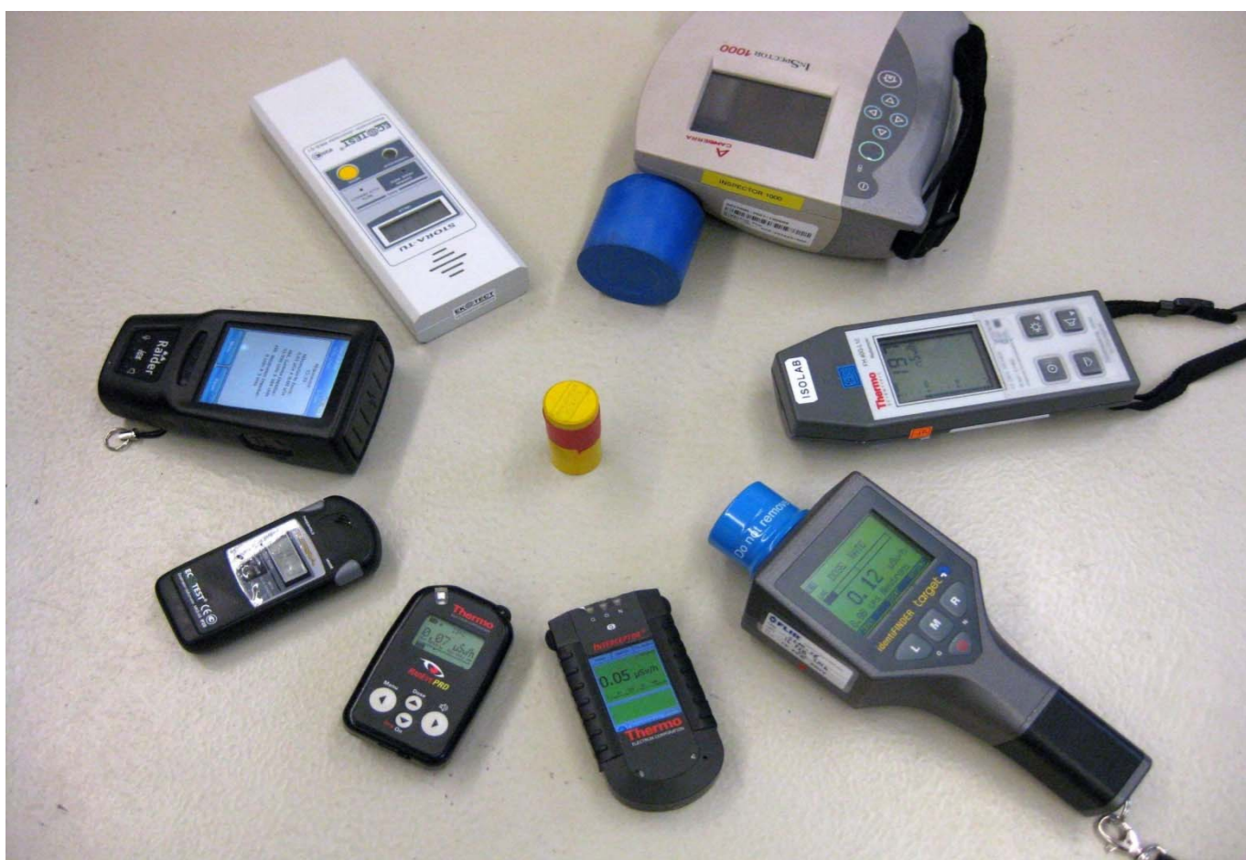
Fig. 1: Measurement setup with hand-held gamma detectors
