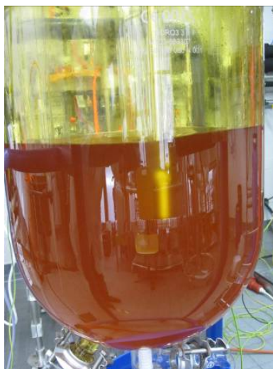
Figure 2: Copolymer ECH/BBrMO in a 30 liter reactor with DMSO and water
