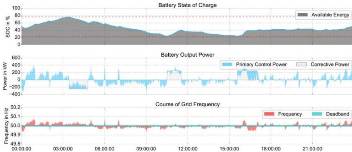
Figure 5: Representative day from the simulation of a BES providing PCR.
