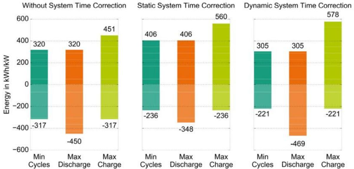
Figure 4: Effects of operation modes and the use of system time correction.
