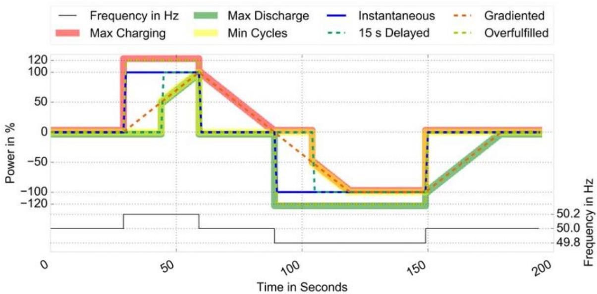
Figure 3: Example PCR power demand with implementation of different degrees of freedom and operation modes.
