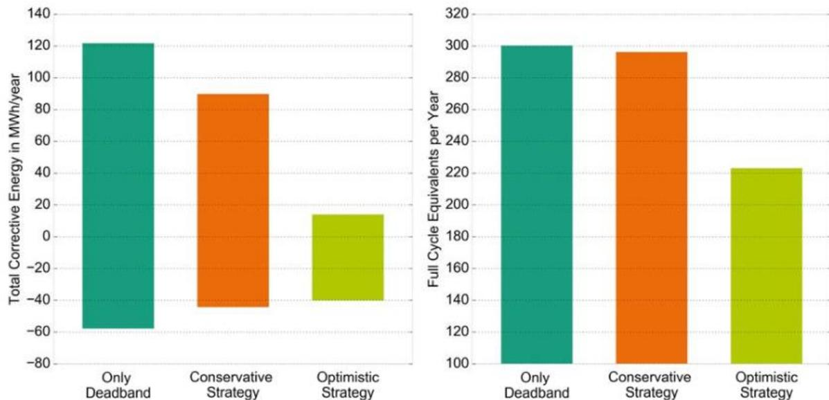
Figure 7: Simulation results of a BES providing PCR using different operation mode implementations.
