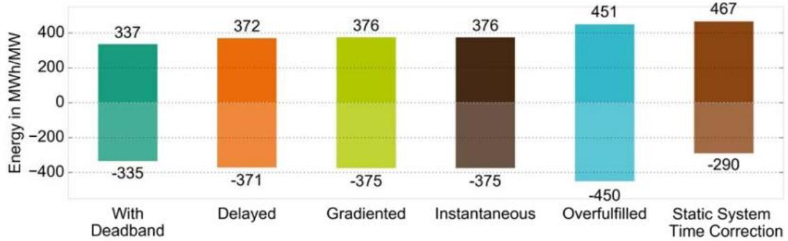
Figure 1. Effects of using each degree of freedom for PCR provision. In the case of BES positive and negative numbers are charging and discharging energy respectively.
