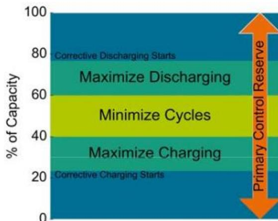
Figure 6: Energy capacity limits for selection operation mode activation.
