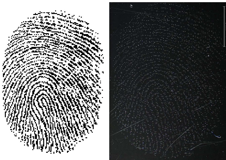
Figure 4: left: Bitmap of a fingerprint, right: result of the printing plotted with \text{KNO}_3
