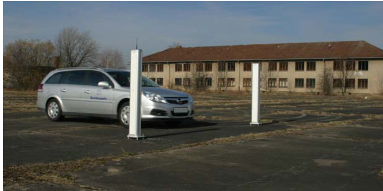
Fig. 1. Car with source inside driving through the portal monitor system.
