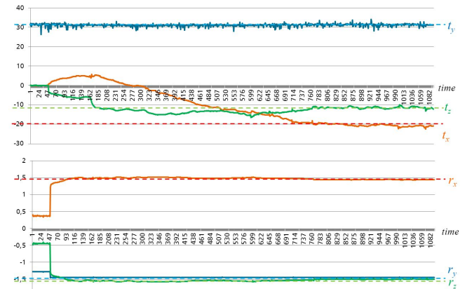
Fig. 7. Resulting extrinsic parameters (top: translation; bottom: rotation). The dotted lines indicate the correct parameter values.
