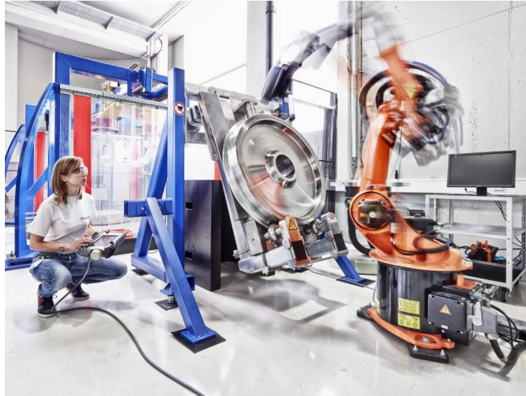
Fig. 10. Demonstrator set-up for surface defect testing on railway wheels by induction thermography using a robot
