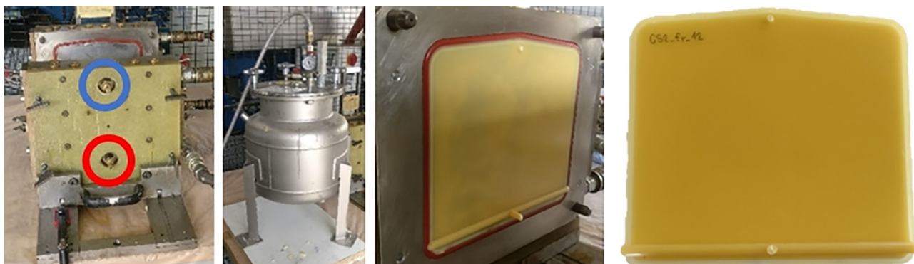
FIGURE 1 Left to right: vertical oriented plate mould with inlet port (red) and vent port (blue); pressure pot which can be connected by a replaceable tube to the inlet port of the plate mould; open mould with cured PUR plate; cured PUR plate
