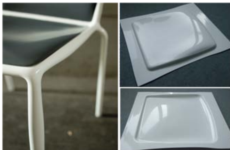
Fig. 14: Powder precoated aluminum blanks formed into parts (right) for a chair (left) by hydroforming.
