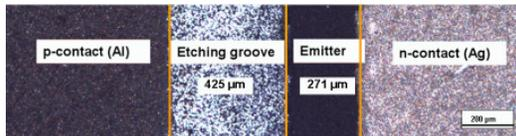
**Figure 9:** Picture of a contact isolation on the rear of a MWT solar cell realized by an etching groove using SolarEtch® SiD. Around 2/3 of the etching groove are visible while one third is covered by aluminum.
