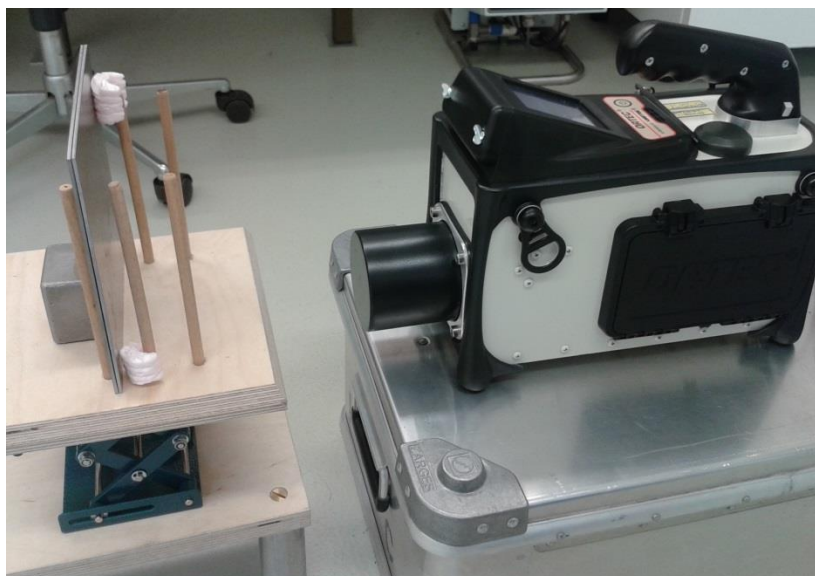
Figure 2: Measurement array with Micro Detective (on the right) and 1.8 kg block of depleted uranium (on the left) shielded by 5 mm of Fe.
