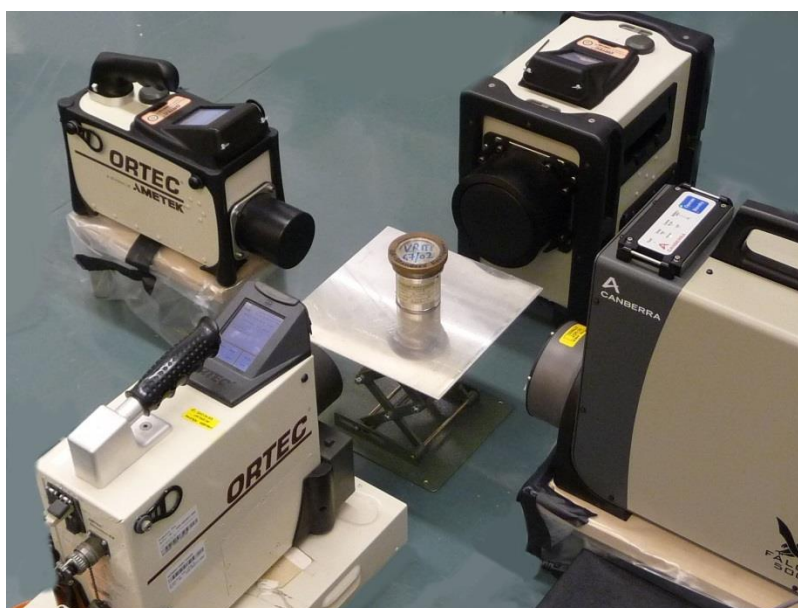
Figure 1: Measurement array with four detectors positioned around an unshielded source; the detectors are (clockwise starting on the bottom left): Detective EX, Micro-Detective, Detective 200 and Falcon 5000.
