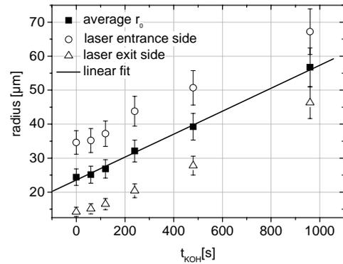
**Figure 5** (Equivalent) radius vs. etching time microscopically measured on both wafer sides. If necessary an equivalent radius was calculated from the area enclosed by a polygon to account for deviations from the circle shape.
