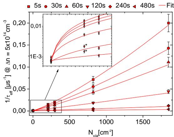
**Figure 7** Inverse  $\tau_{\text{eff}}$  vs.  $N_{\text{via}}$  for different etching times with fits according to Opdorp et al. for SiN layer. Recombination decreases with etching time as well as decreasing via-hole density. The extracted  $S_{\text{via}}$  ranges from 18200cm/s to 60cm/s (Table 1).
