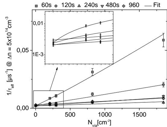
**Figure 8** Inverse  $\tau_{\text{eff}}$  vs.  $N_{\text{via}}$  for different etching times with fits according to Opdorp et al. for SiO layer. The values of  $S_{\text{via}}$  of the oxide samples is about half of the values of the SiN-samples.
