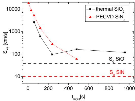
**Figure 9**  $S_{\text{via}}$  values extracted from fits vs. etching time for both sample types. For the  $\text{SiO}$ -samples saturation for  $t_{\text{KOH}}$  equal or greater can be observed. The  $\text{SiN}$ -samples show lower values up to 240s indicating the radius-dependence of the passivating effect.
