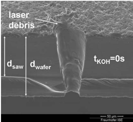
**Figure 2** Cross section of via-hole in Cz-wafer after drilling. Laser debris is present on the surface. The via-hole wall appears to be smooth.
