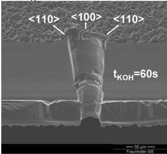
**Figure 3** Cross section of via-hole in Cz-wafer after  $t_{KOH}=60s$ . The anisotropy of the alkaline etch is visible.
