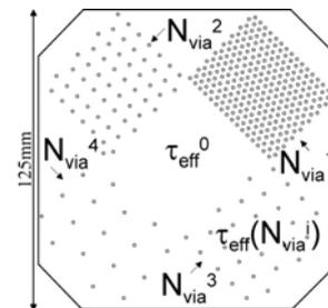
**Figure 1** Lifetime sample design.  $\tau_{\text{eff}}(N_{\text{via}}^i)$  is measured on 4 areas of different via-density surrounding a reference area without via-holes.
