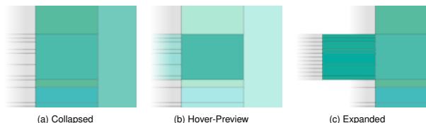
Fig. 6: Example code hierarchy section with visible expand indicators. (a) shows the hierarchy collapsed to class-level. In (b), a hovered class member function indicators are highlighted, to be expanded by a click-interaction. (c) shows the result of the click.
