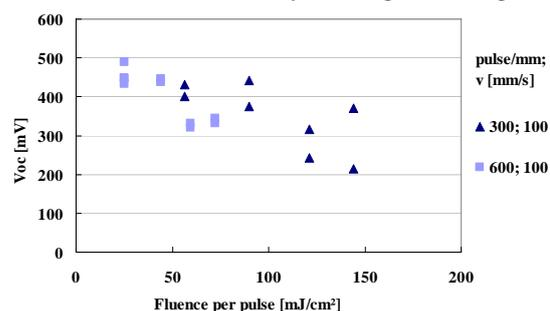
**Fig. 2:** Suns-Voc measurements of silicon solar cells contacted by laser melting process of titan nitride
