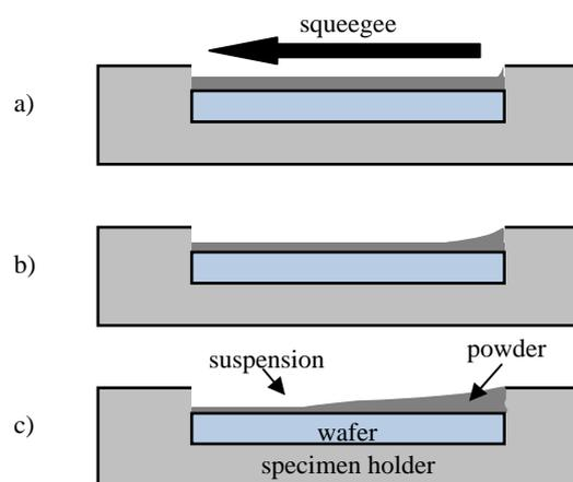
**Fig. 6:** Different coating distributions depending on the time between depositing a suspension on the edge of the specimen holder and spreading it: a) fast, b) medium, c) slow
