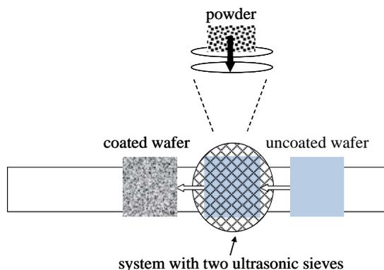
**Fig. 5:** Configuration of the two ultrasonic sieve techniques
