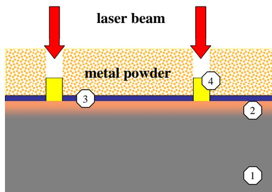
**Fig. 1:** Deposition of a seed layer by a laser beam
