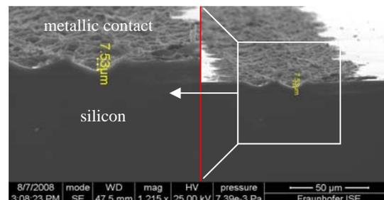
**Fig. 3:** Influence of the powder roughness for depth damage shown by SEM. Laser parameters (Nd:YAG 1064 nm, 8000 Pulses/mm, pulse energy density: 8.42 mJ/cm²). Powder: TiN
