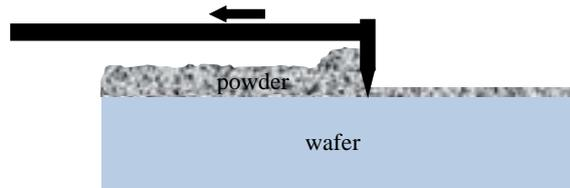
**Fig. 4:** A squeegee dispenses powder on top of a wafer
