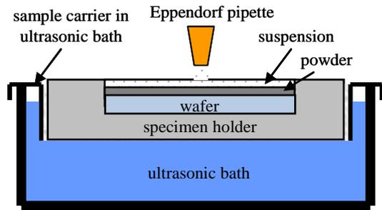
**Fig. 7:** Configuration for an ultrasonic dryer of a suspension
